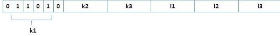
Figure 3.2 – Visualization of the chromosome structure used for the Hawai'iSat-1 gain tuning problem.
